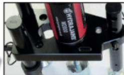
Improved load spreading bridge design.
